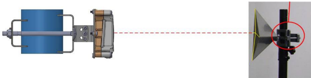
Figure 5.1: Mounting alignment of radar and reflector
