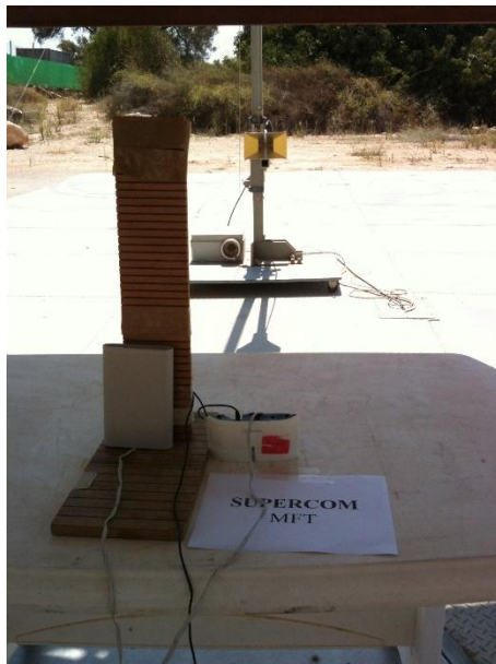
Radiated Emission Test – External Antenna
