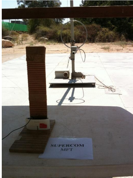
Radiated Emission Test – Internal Antenna
