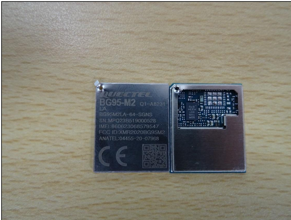
RF Module with shield removed
