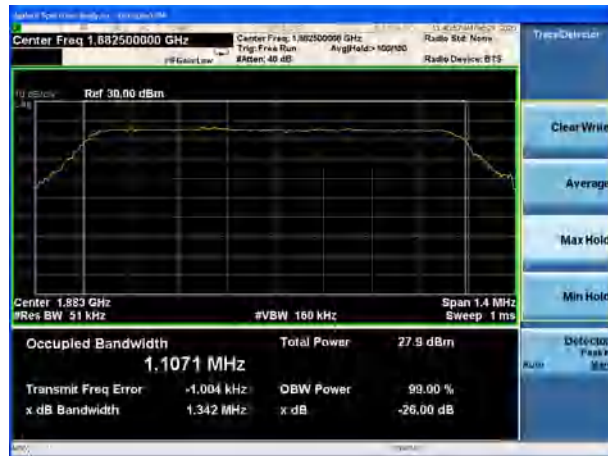
LTE Band 25 5MHz QPSK CH-Middle
