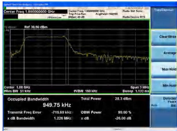
LTE Band 2 10MHz 16QAM CH-Middle
