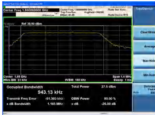
LTE Band 2 5MHz 16QAM CH-Middle
