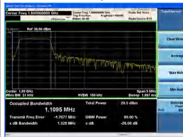
LTE Band 2 15MHz QPSK CH-Middle
