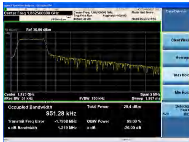
LTE Band 25 15MHz 16QAM CH-Middle
