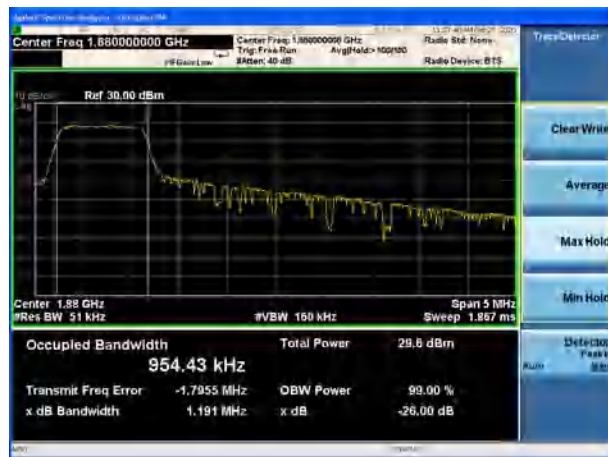
LTE Band 2 15MHz 16QAM CH-Middle
