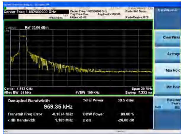
LTE Band 25 20MHz 16QAM CH-Middle
