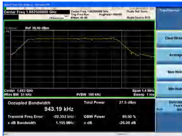
LTE Band 25 5MHz 16QAM CH-Middle
