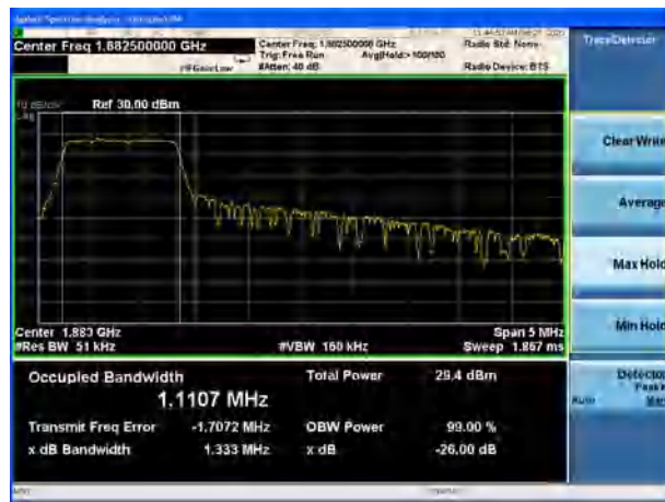
LTE Band 25 15MHz QPSK CH-Middle
