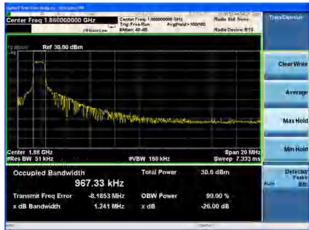
LTE Band 2 20MHz 16QAM CH-Middle
