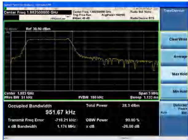
LTE Band 25 10MHz 16QAM CH-Middle
