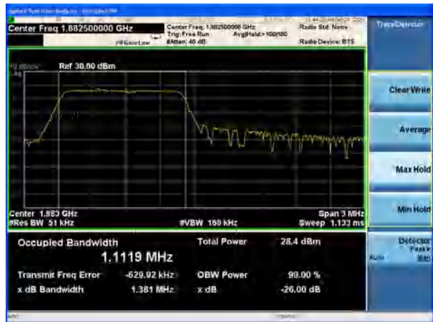
LTE Band 25 10MHz QPSK CH-Middle
