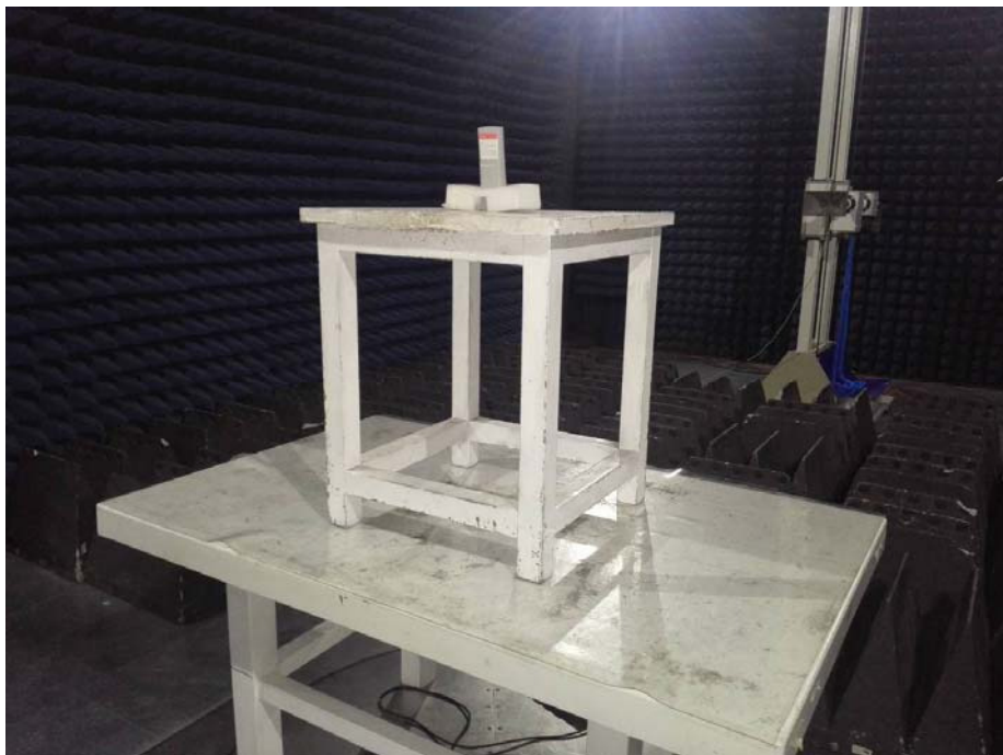
Test frequency above 1GHz at test site 1#
