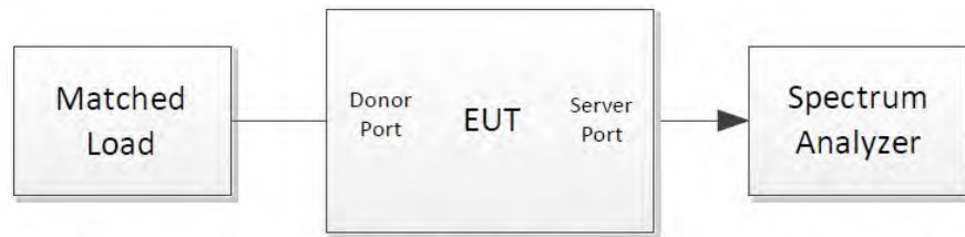
Figure 6 – Maximum downlink noise limit test configuration
