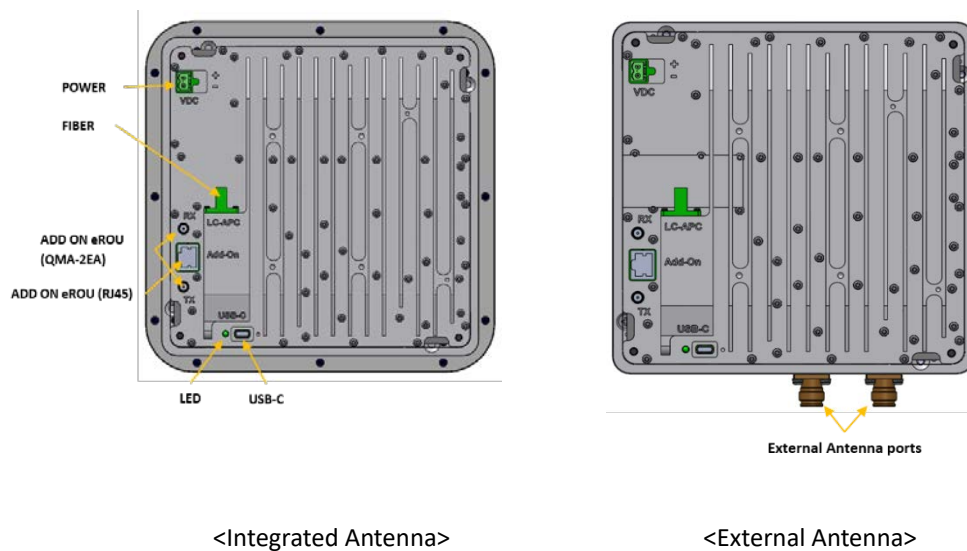
Figure 4. The name of each port on eROU
