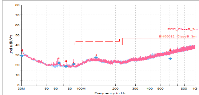
Figure B3: Radiated Emissions 30M-1G Hz for FCC/ISED - 120V/60H - TX Worst-Case
