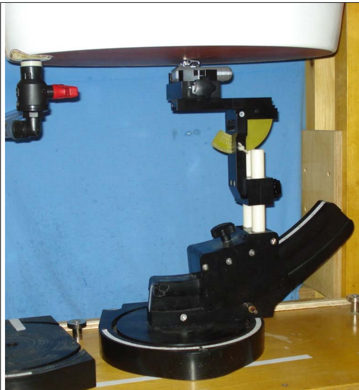
Body-worn SAR Configuration Test Setup with Belt-Clip
