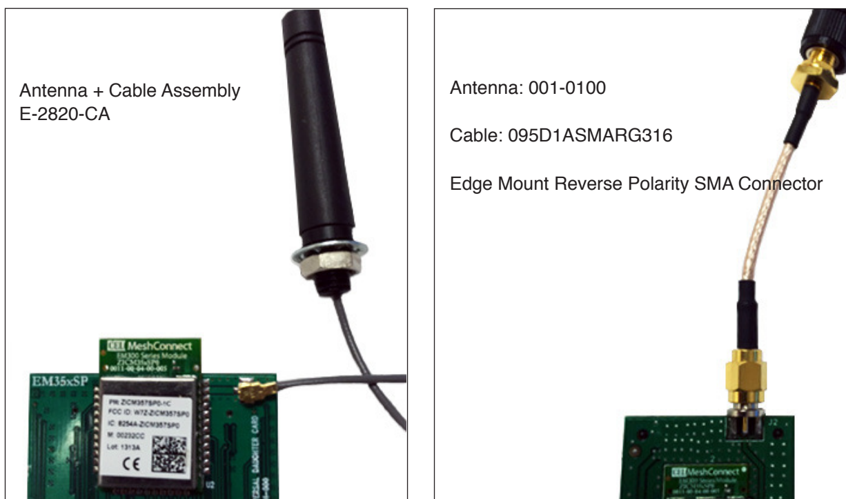
Figure 3. Implementation using connector, cable and external antenna
