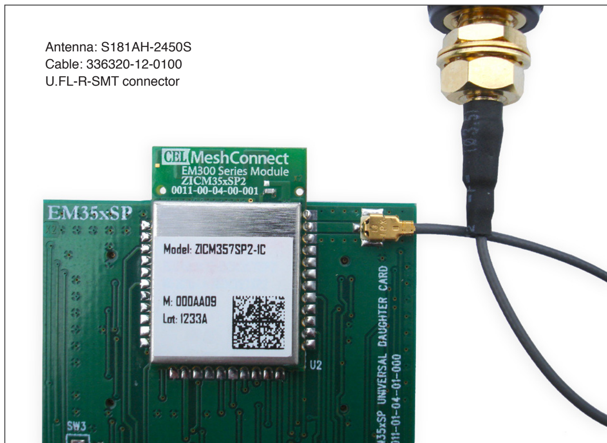
Figure 4. Implementation using connector, cable and external antenna
