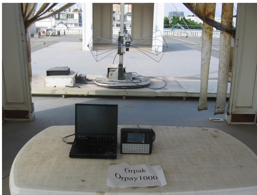
Figure 5. Radiated Emission 30MHz-200MHz
