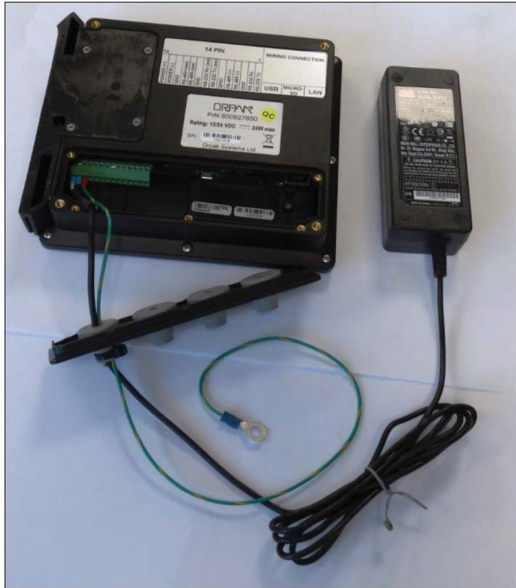
Figure 2-11 - Ground Cable Connected to OrPAY1000
