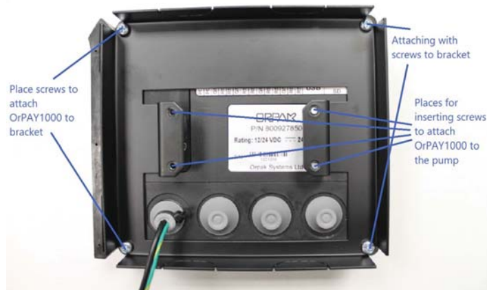
Figure 2-3 - OrPAY1000 Tightened to Bracket
