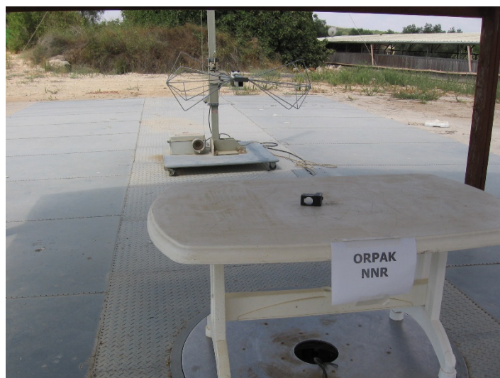
Figure 4. Radiated Emission Test Setup 2.4 GHz
