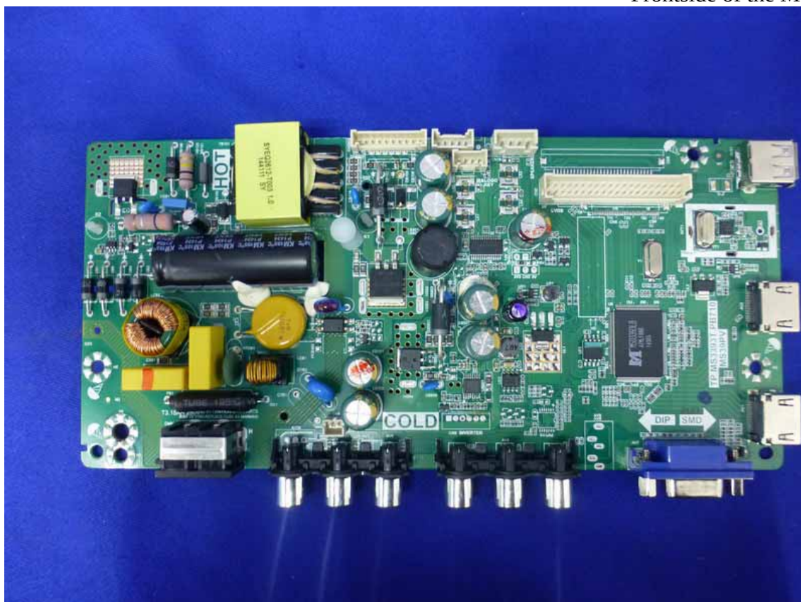
Figure 15 Frontside of the Main Board
