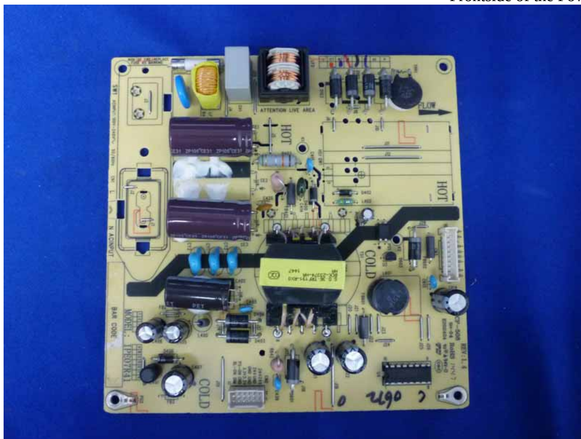
Figure 21 Frontside of the Power Board
