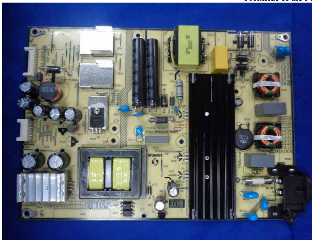
Figure 11 Frontside of the Power Board
