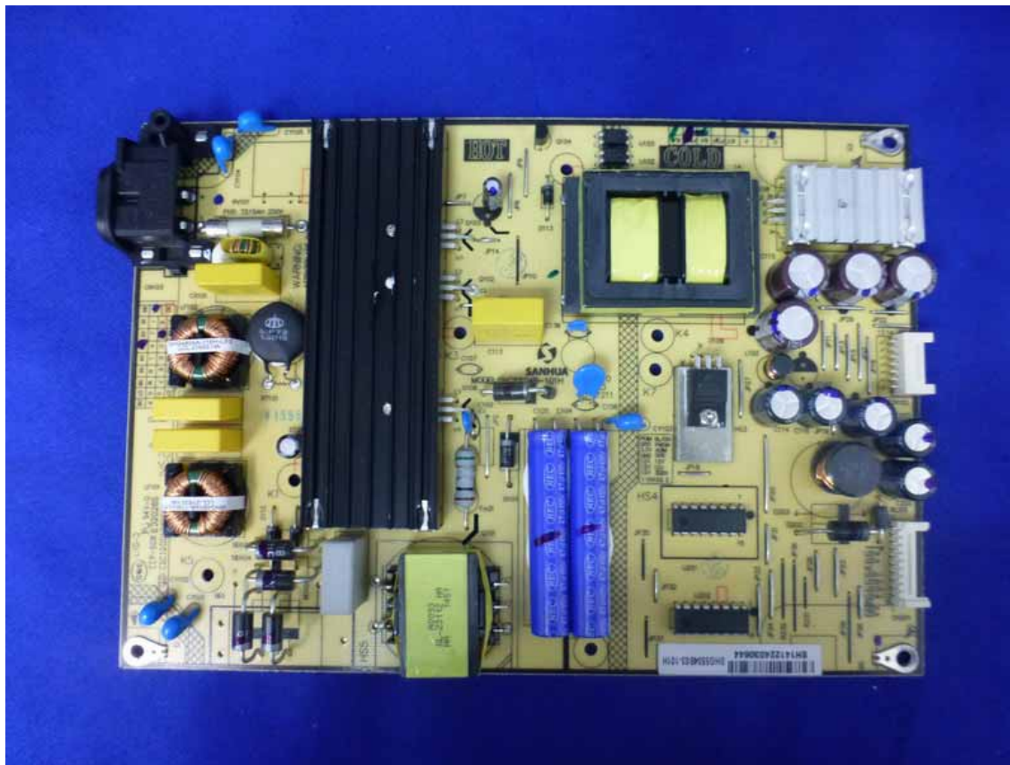
Figure 13 Frontside of the Power Board
