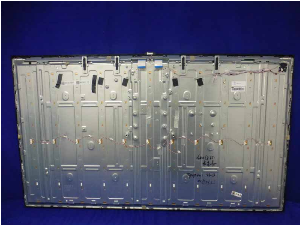
Figure 11 Backside of the LCD Panel
