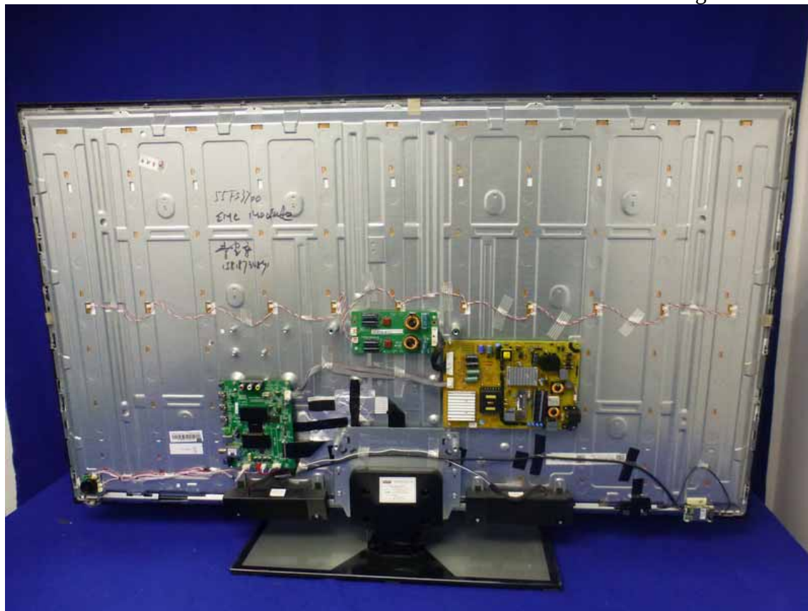
Figure 7 Inside Configuration of the EUT
