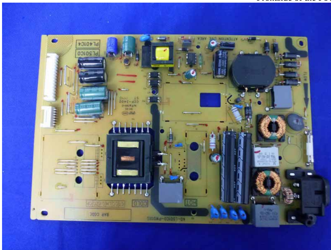
Figure 19 Frontside of the Power Board
