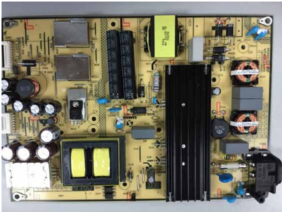
Figure 13 Frontside of the Power Board
