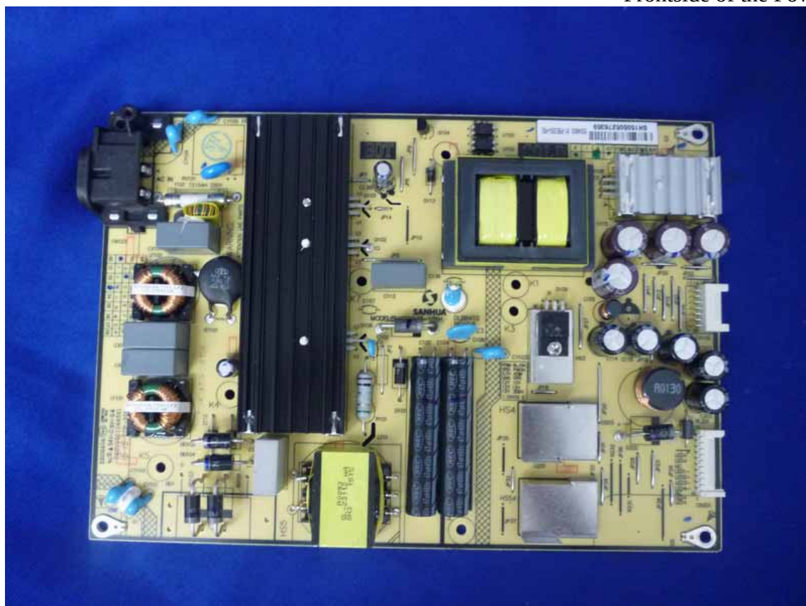
Figure 10 Frontside of the Power Board
