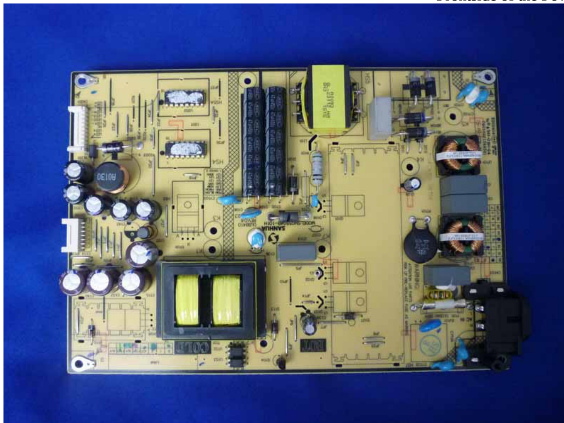
Figure 12 Frontside of the Power Board
