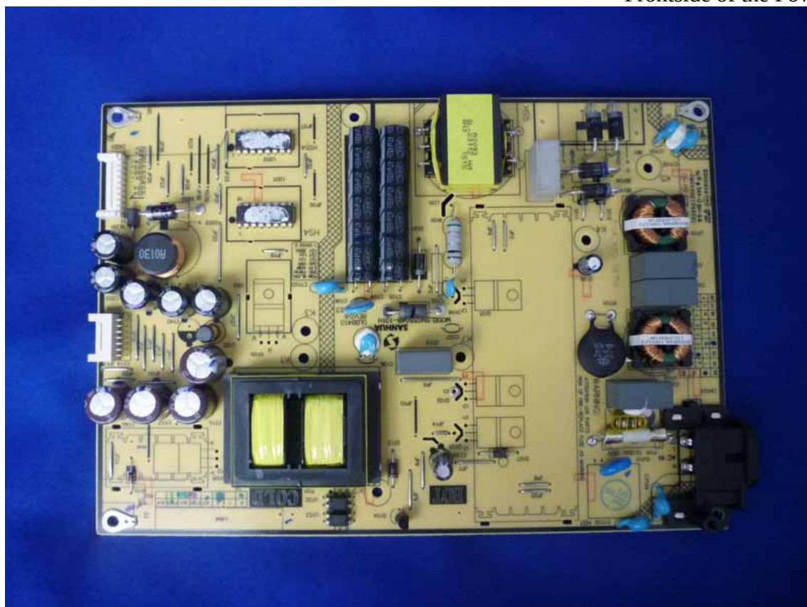
Figure 11 Frontside of the Power Board
