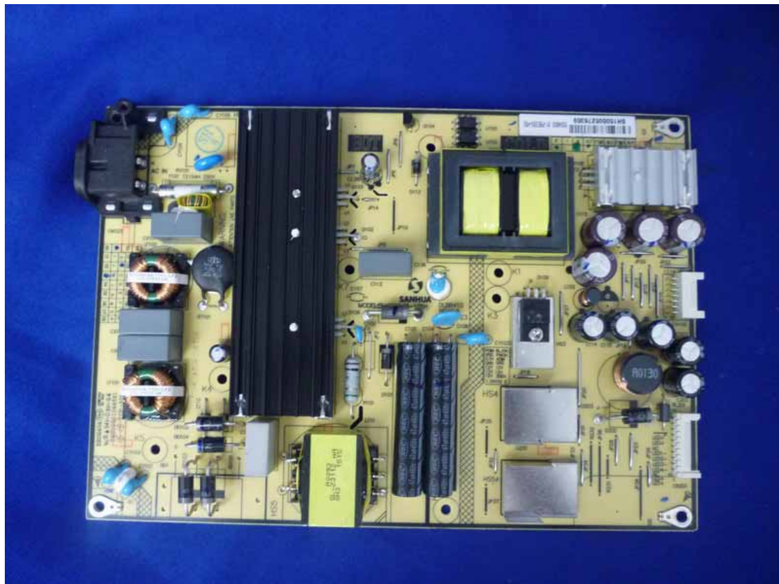
Figure 9 Frontside of the Power Board
