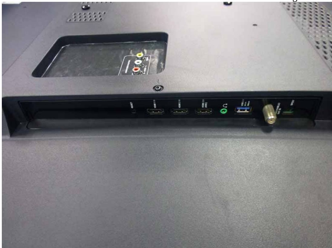
Figure 6 Signal Port of the EUT
