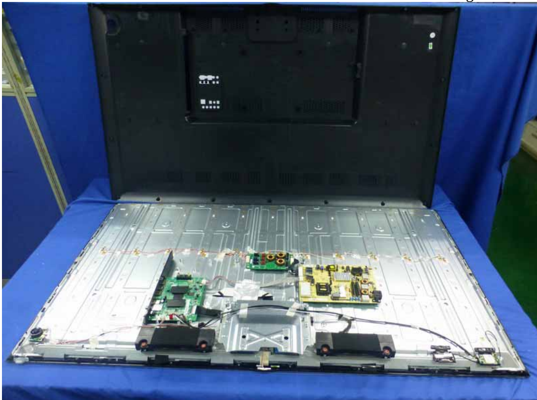
Figure 8 Inside Configuration of the EUT
