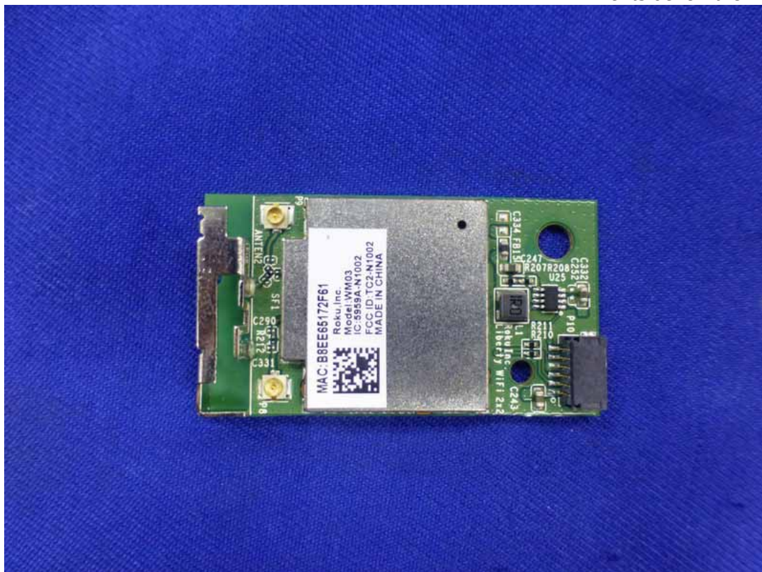
Figure 26 Frontside of the PCB Board
