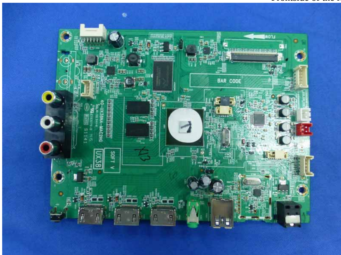
Figure 14 Frontside of the Main Board
