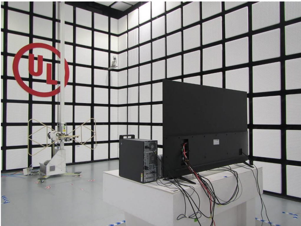
Radiated Disturbance below 1GHz – rear view
