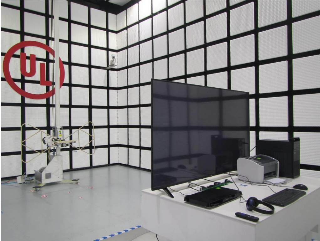
Radiated Disturbance below 1GHz – front view
