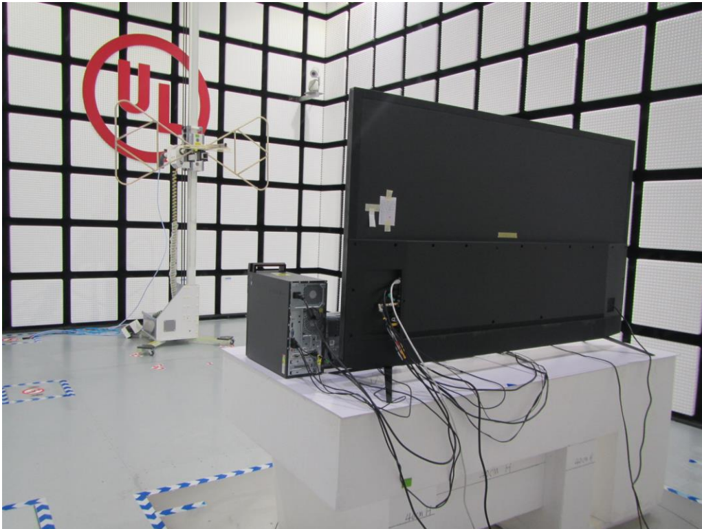
Radiated Disturbance below 1GHz – rear view
