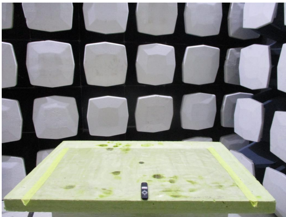
Below 1GHz: EUT is placed on the center of the turn table
