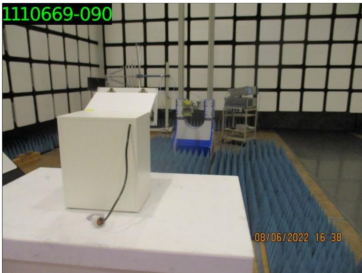
42 Picture 3: Radiated disturbance (> 1 GHz)
