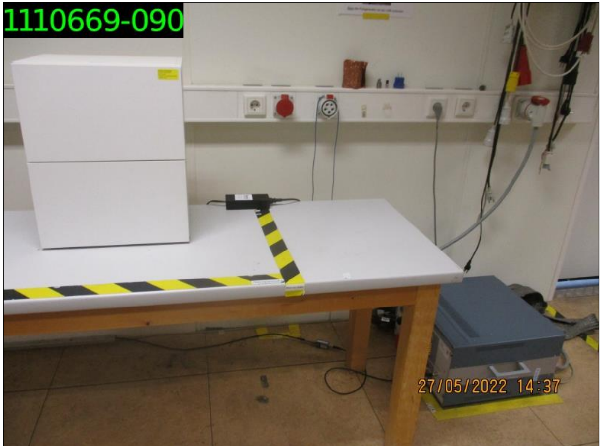
41 Picture 2: Conducted voltage emissions
