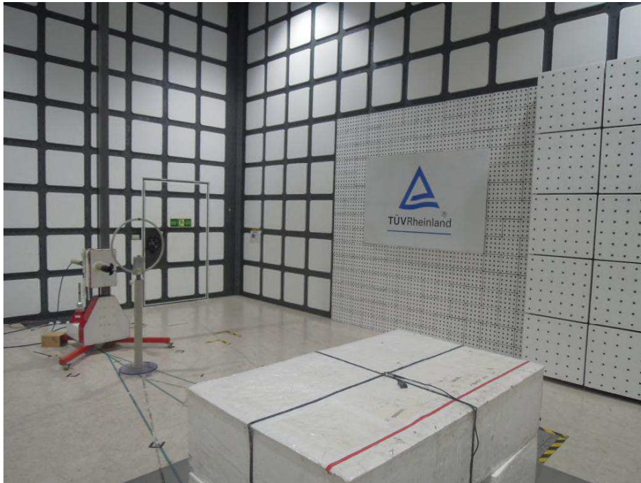
Photograph 6: Set-up for Spurious Emissions (Back View 4)
