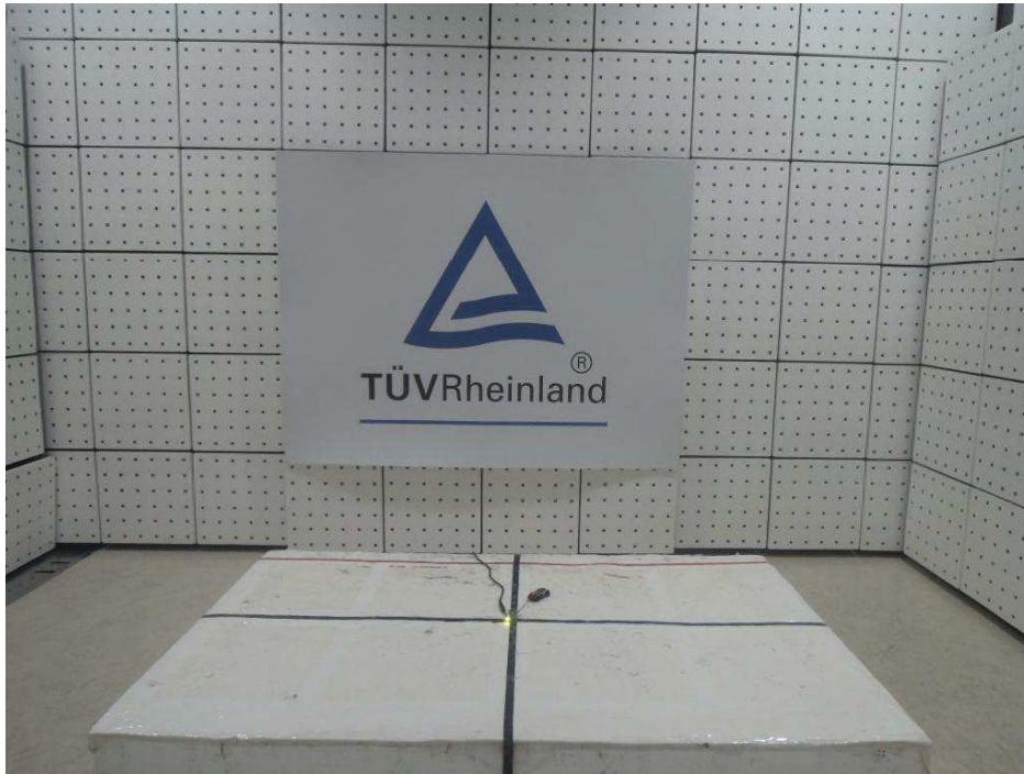
Photograph 2: Set-up for Spurious Emissions (Front View 2)
