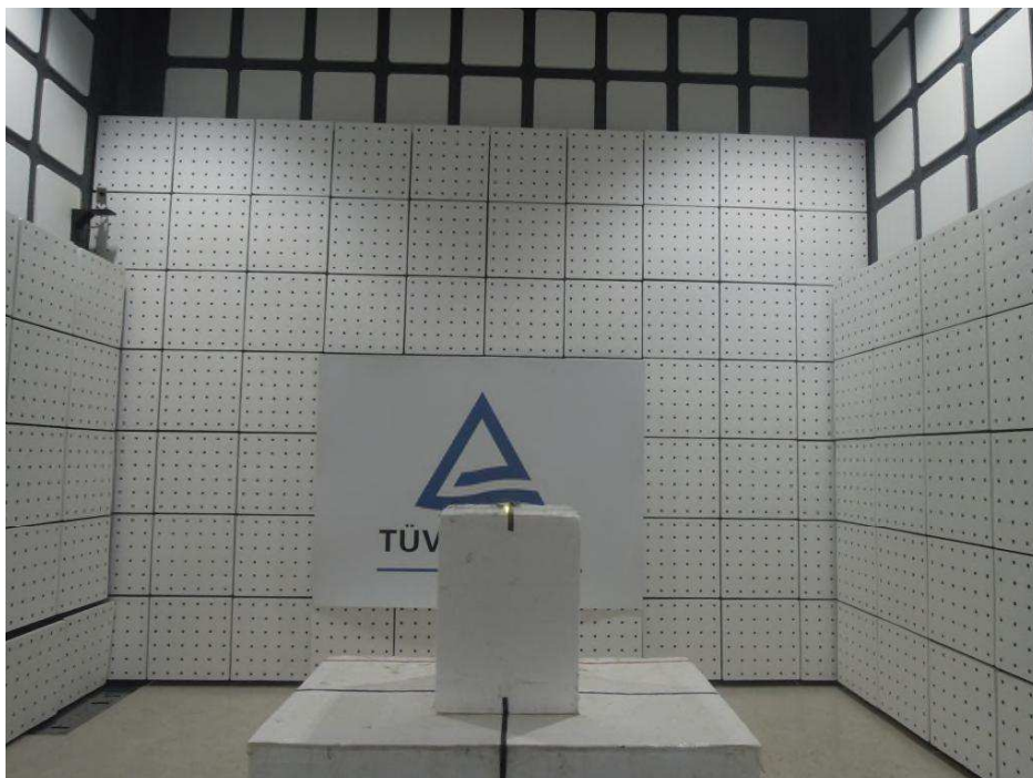
Photograph 2: Set-up for Spurious Emissions (Front View 2)
