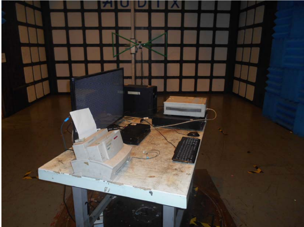
SETUP WITH MAXIMUM DETECTED EMISSION AT HORIZONTAL POLARIZATION (TEST MODE: USB PLAY)
