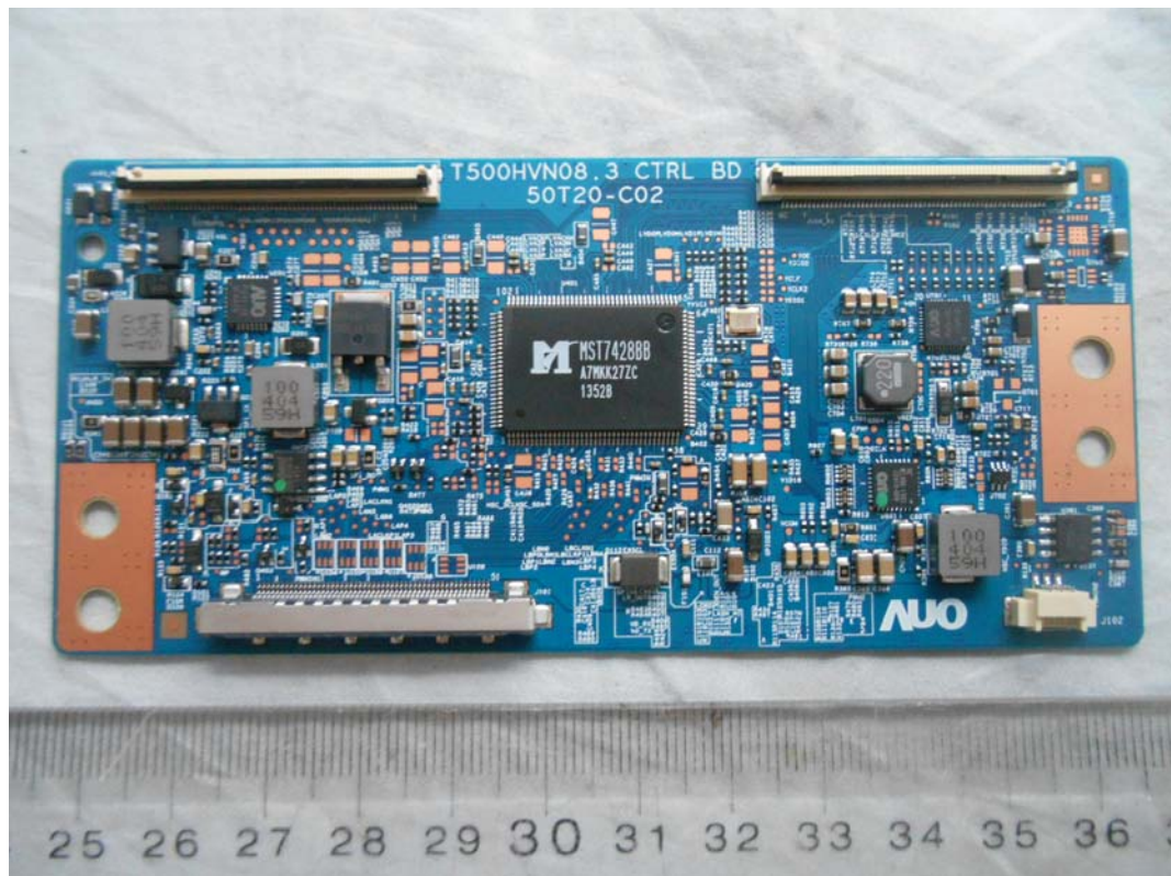
FIGURE 17 LED LCD TV (M/N: 50H7EG) LCD PANEL CONTROL BOARD (COMPONENT SIDE)
