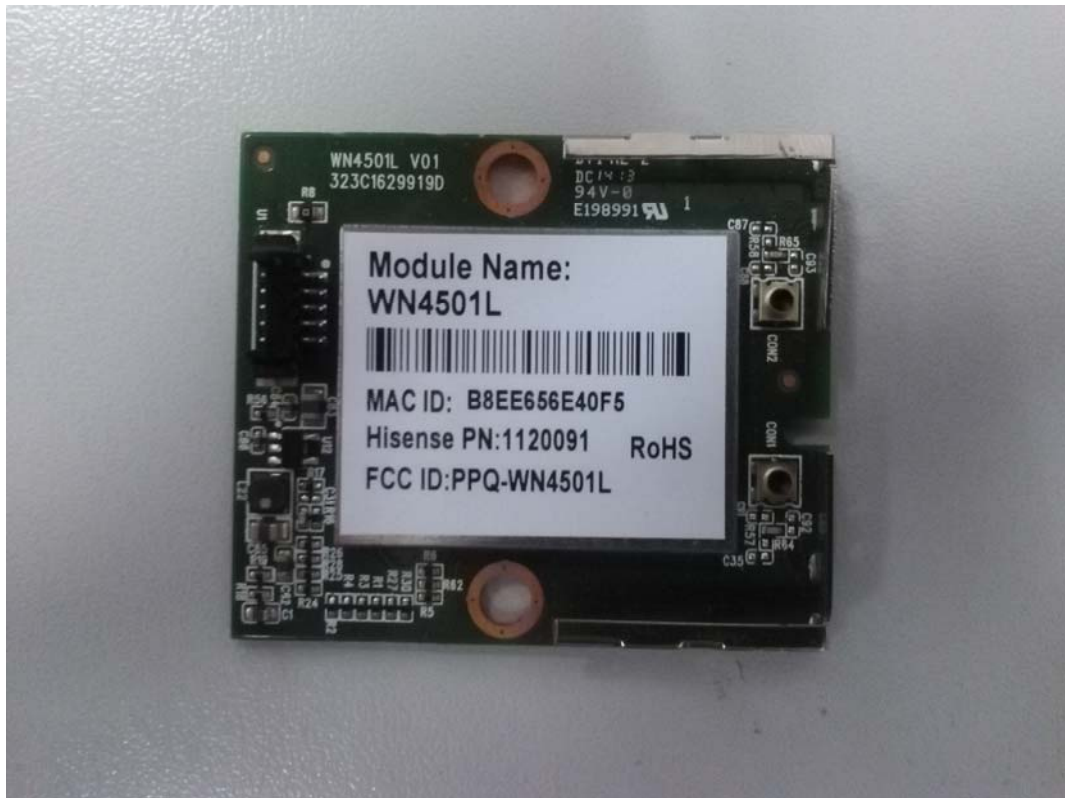
FIGURE 15 LED LCD TV (M/N: 50H7EG) RF BOARD #2 (COMPONENT SIDE)
