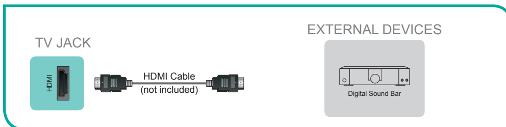
Figure 13. Digital Sound Bar to the HDMI (ARC) port
