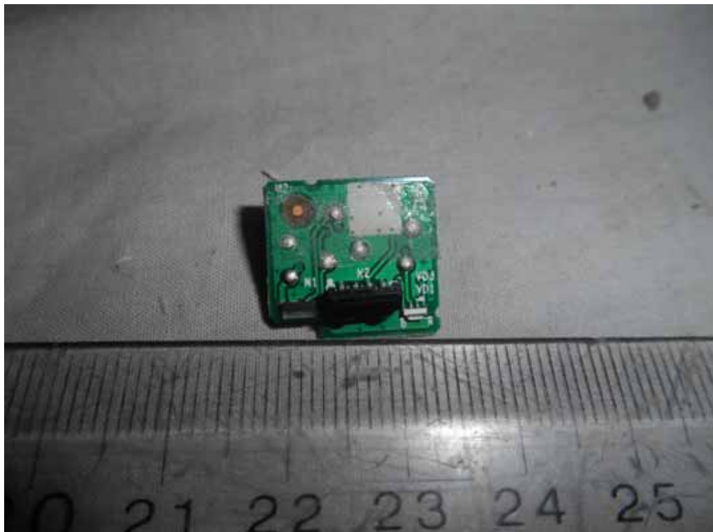
FIGURE 20 LED LCD TV (M/N: PLDED6079-SM) IR BOARD (COMPONENT SIDE)
