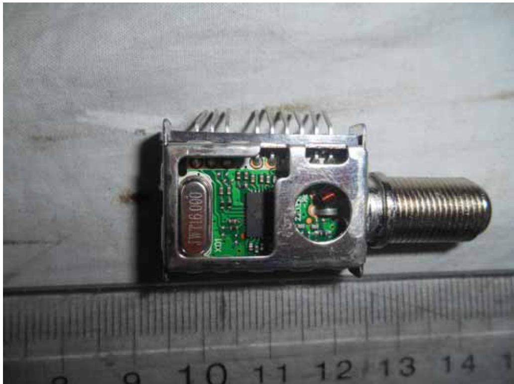
FIGURE 7 LED LCD TV (M/N: PLDED6079-SM) TUNER BOARD (COMPONENT SIDE)
