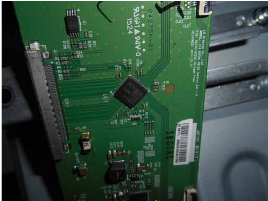
FIGURE 15 LED LCD TV (M/N: PLDED6079-SM) CHIP AND CRYSTAL ON PANEL BOARD
