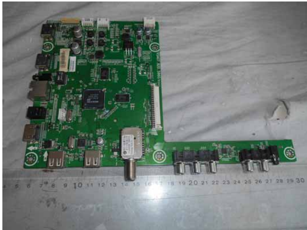
FIGURE 3 LED LCD TV (M/N: PLDED6079-SM) MAIN BOARD (COMPONENT SIDE)
