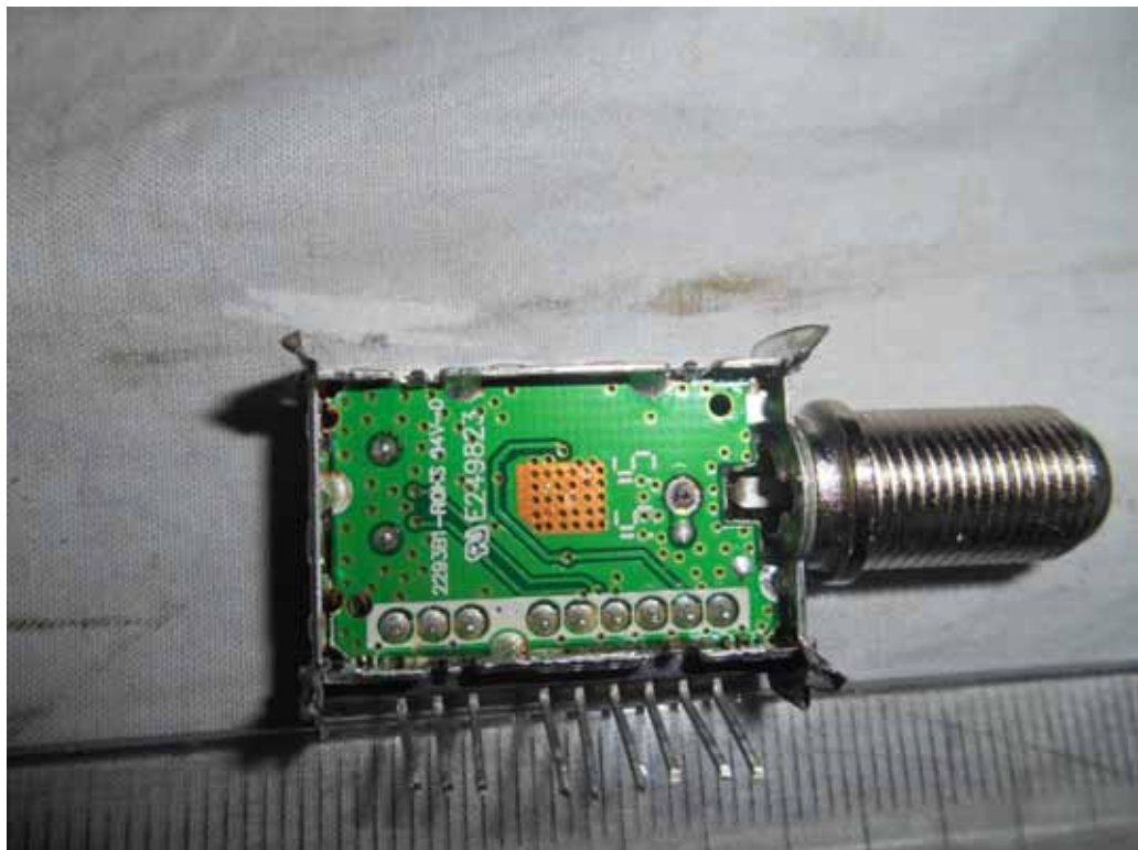
FIGURE 8 LED LCD TV (M/N: PLDED6079-SM) TUNER BOARD (SOLDERED SIDE)
