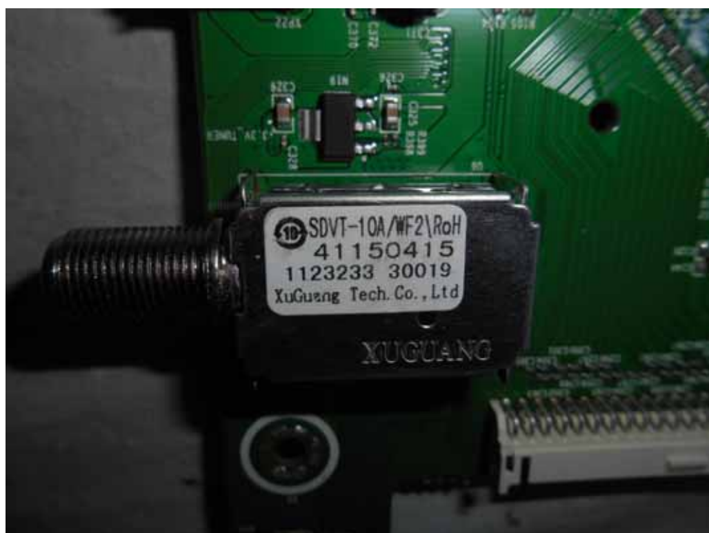
FIGURE 6 LED LCD TV (M/N: PLDED6079-SM) TUNER
