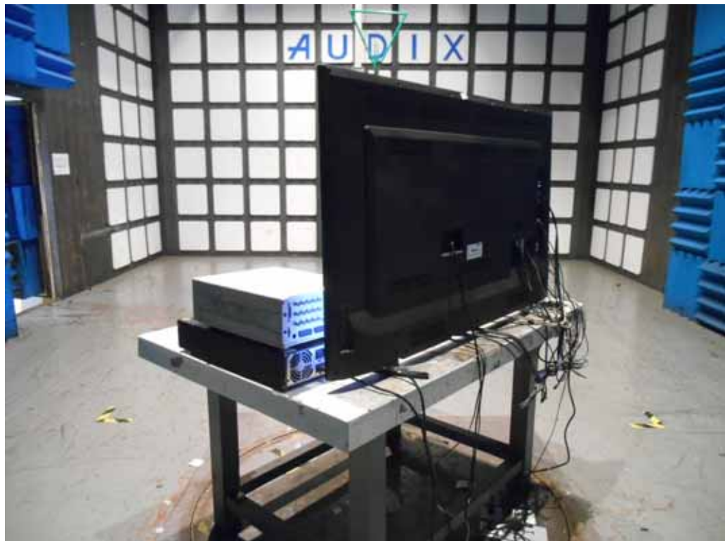
SETUP WITH MAXIMUM DETECTED EMISSION AT VERTICAL POLARIZATION (TEST MODE: HDMI 1024*768@60Hz & 1kHz Playing)
