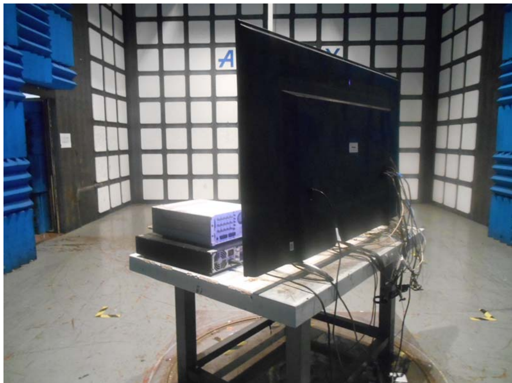
SETUP WITH MAXIMUM DETECTED EMISSION AT VERTICAL POLARIZATION (TEST MODE: HDMI1080P)
