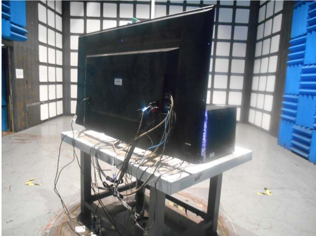
SETUP WITH MAXIMUM DETECTED EMISSION AT HORIZONTAL POLARIZATION (TEST MODE: HDMI1080P)
