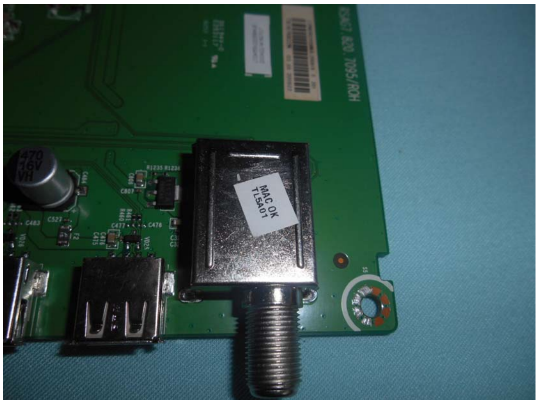
FIGURE 8 LED LCD TV (M/N: LC-55F) TUNER
