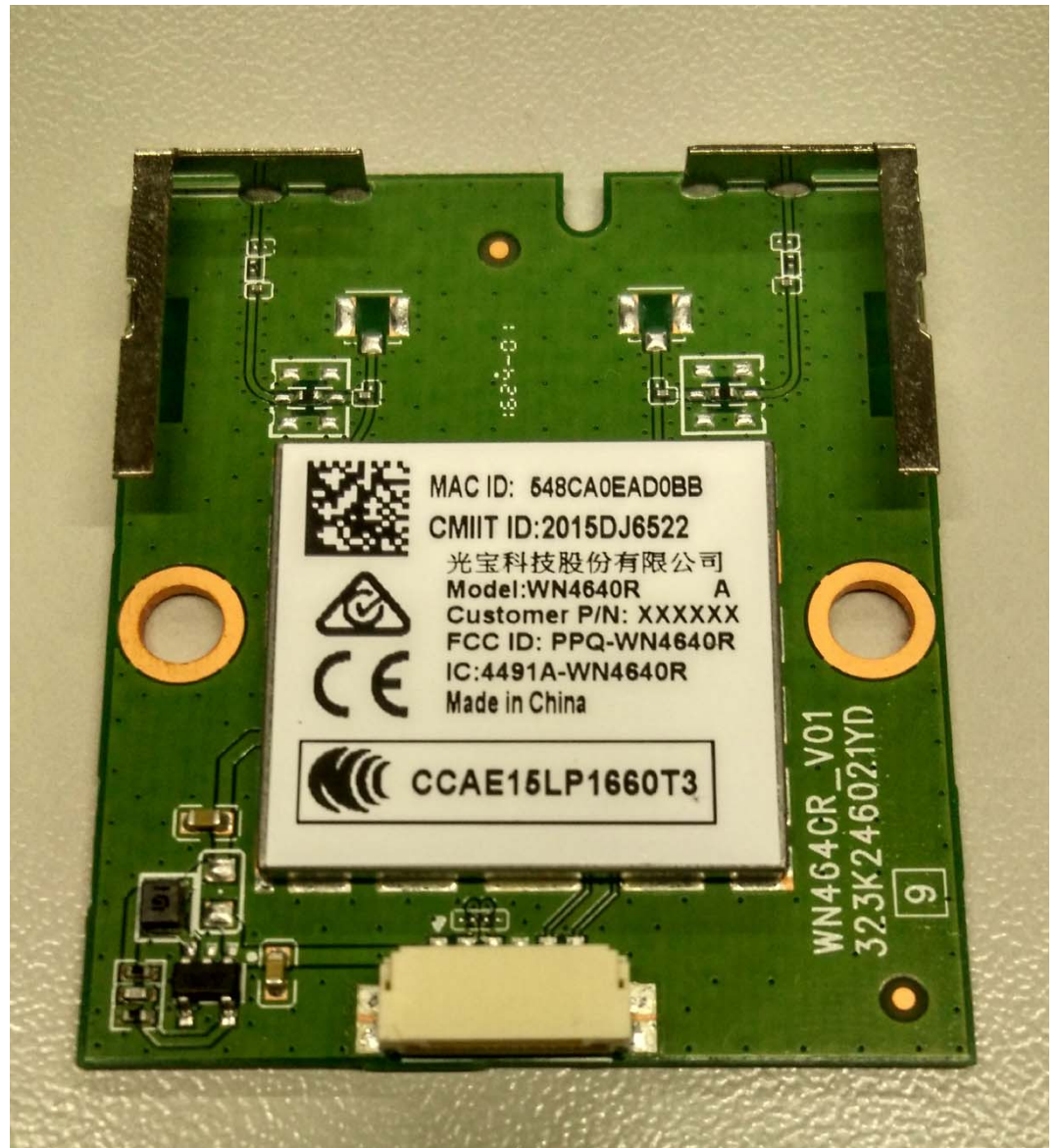
FIGURE 19 LED LCD TV (M/N: LC-55F) RF BOARD LABEL
