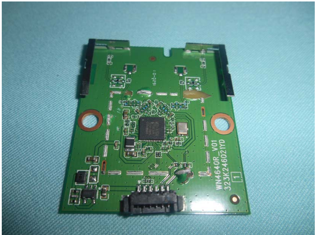
FIGURE 20 LED LCD TV (M/N: LC-55F) CHIP AND CRYSTAL ON RF BOARD
