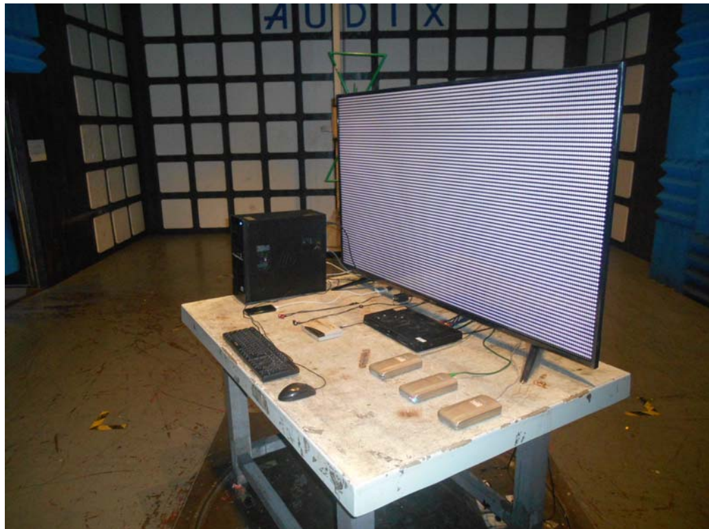
SETUP WITH MAXIMUM DETECTED EMISSION AT VERTICAL POLARIZATION (TEST MODE: HDMI1 3840*2160@60Hz & 1kHz PLAYING)
