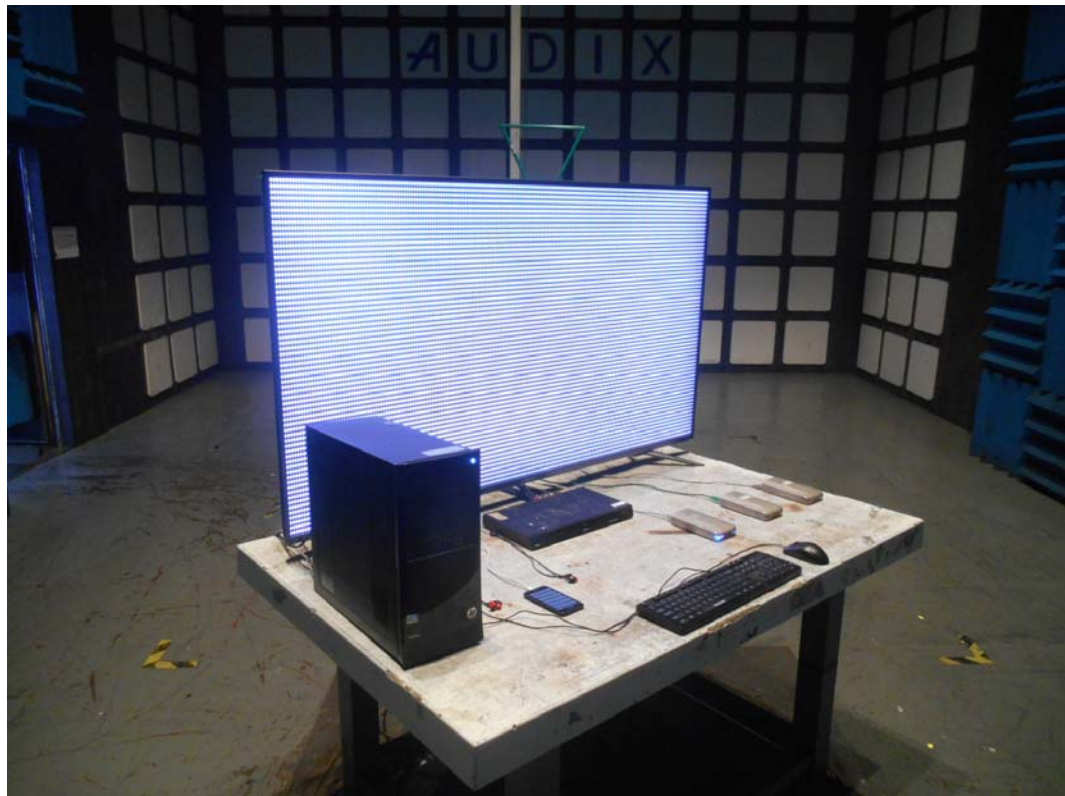
SETUP WITH MAXIMUM DETECTED EMISSION AT VERTICAL POLARIZATION (TEST MODE: HDMI2 3840*2160@60Hz & 1kHz PLAYING)
