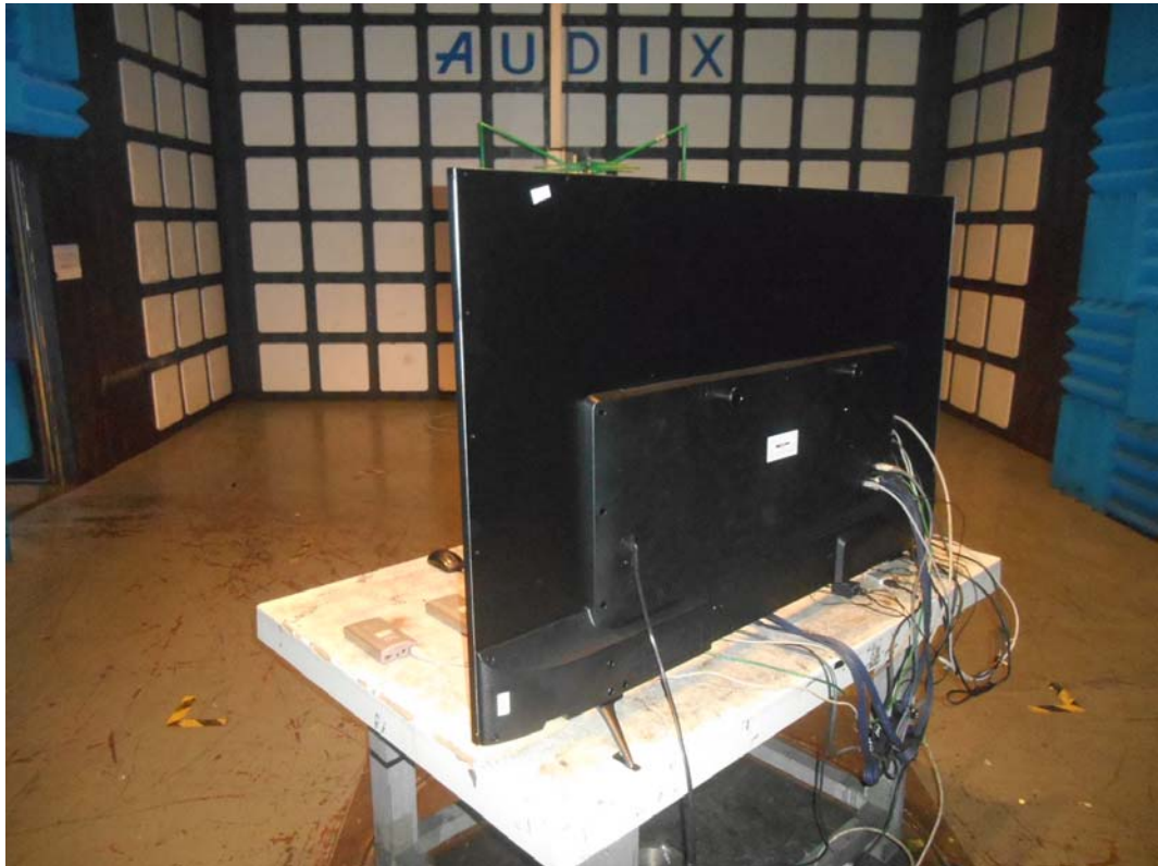
SETUP WITH MAXIMUM DETECTED EMISSION AT HORIZONTAL POLARIZATION (TEST MODE: HDMI2 3840*2160@60Hz & 1kHz PLAYING)
