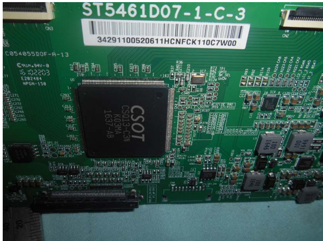
FIGURE 17 LED LCD TV (M/N: 55R6D) CHIP AND CRYSTAL ON PANEL BOARD
