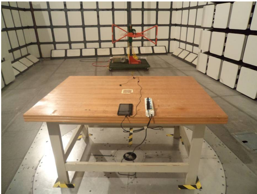
Radiated Emissions - Rear View (Below 1 GHz)
