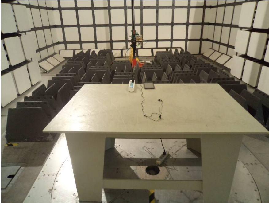
Radiated Emissions – Front View (Above 1 GHz)
