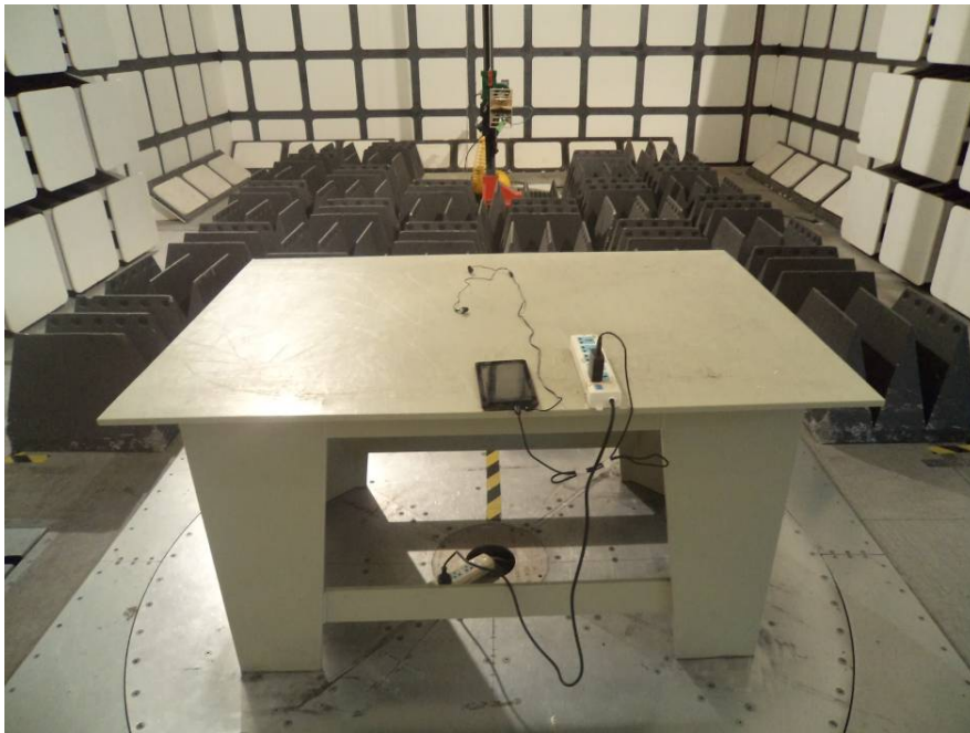
Radiated Emissions – Rear View (Above 1 GHz)
