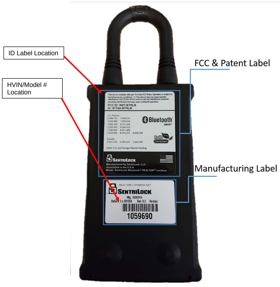
Photograph 4: Label Locations (Label Text Not Specific to this Device)
