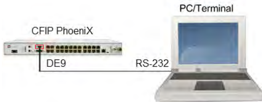
Figure 2.14 Serial connection to CFIP Phoenix
