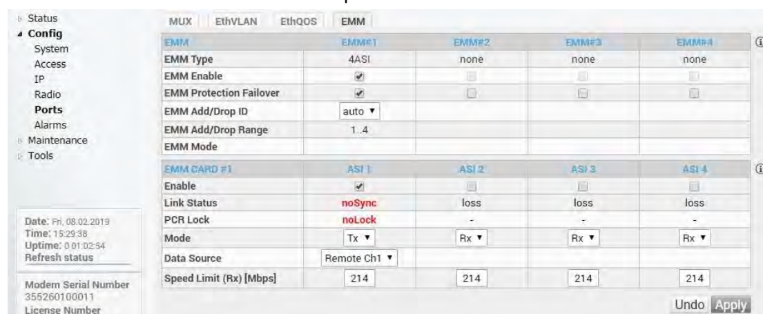
Figure 5.95 Example of Side B Secondary IDU EMM configuration
