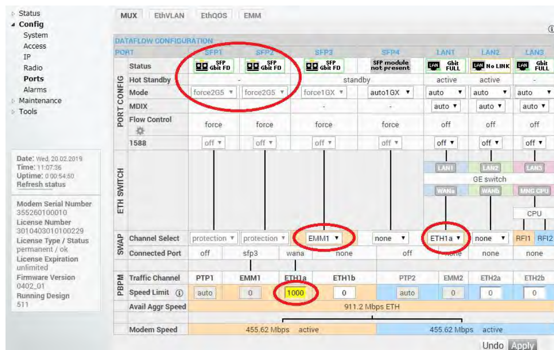
Figure 5.127 Example of port configuration
