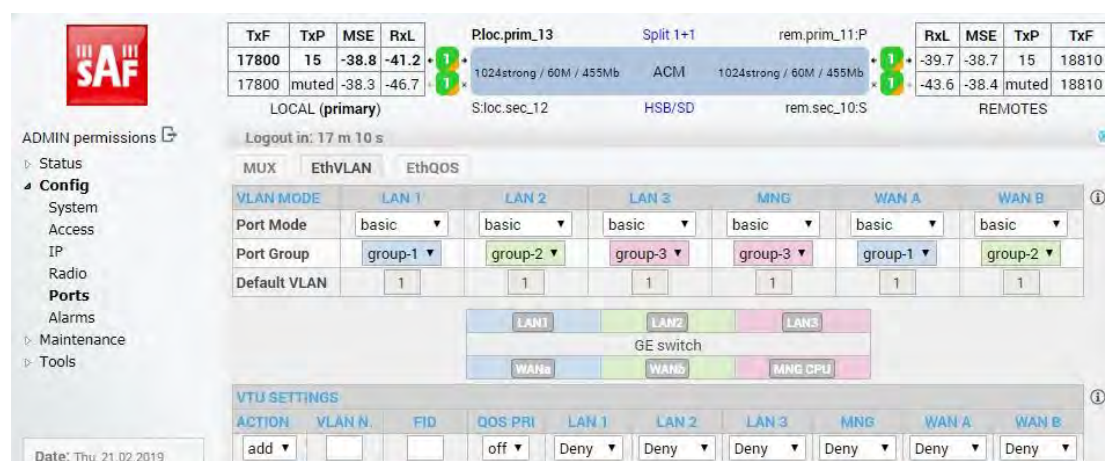
Figure 5.147 Example of port grouping
