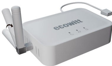
Figure 3 Lock and Adjust the Angle
