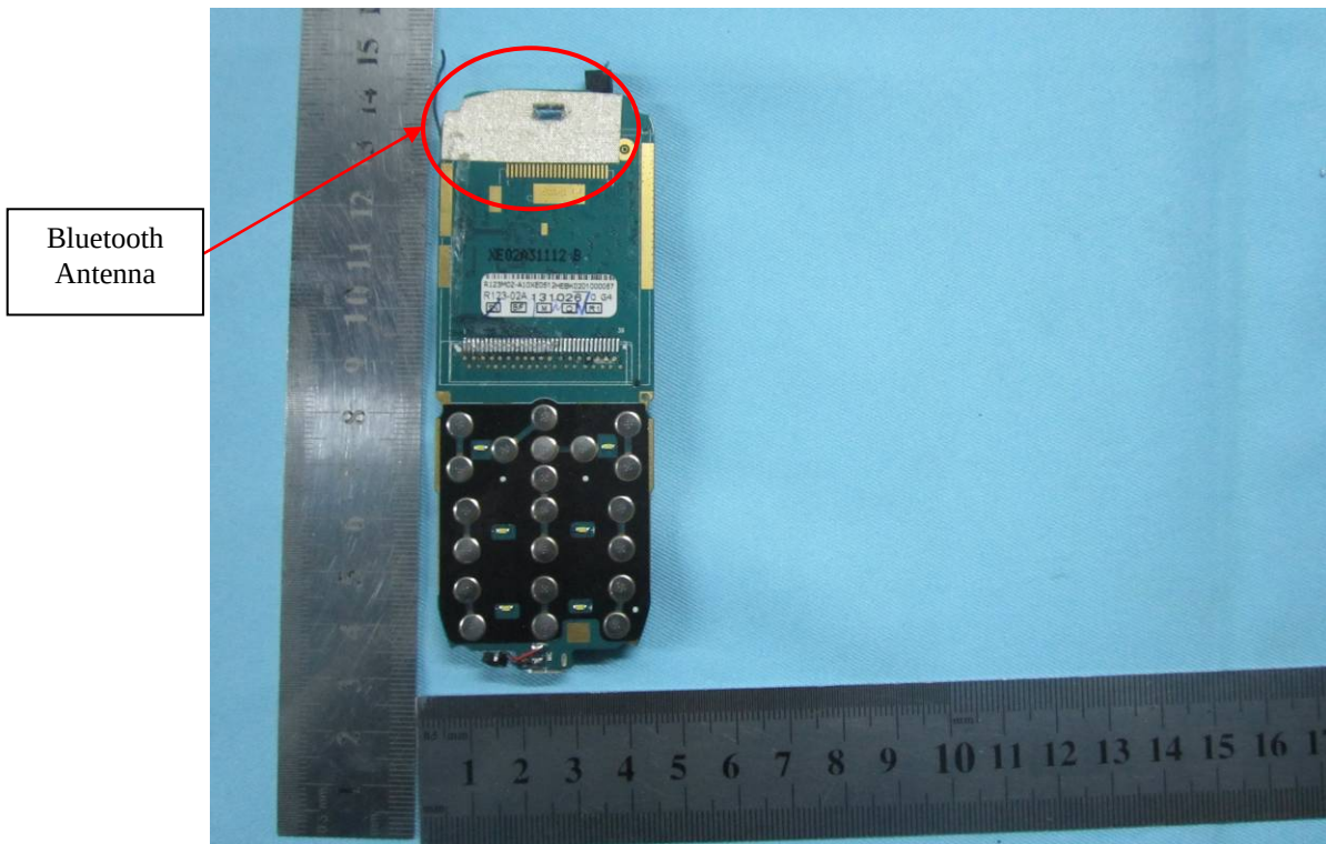
Mainborad With Shielding - Rear View
