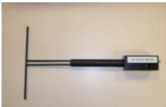
Figure 1 – Satimo COMOSAR Validation Dipole
