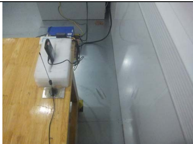
Conducted Emissions Test Setup Side View
