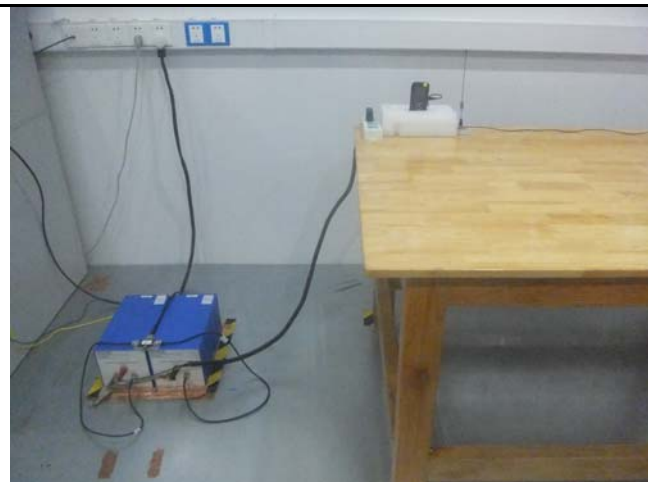
Conducted Emissions Test Setup Front View
