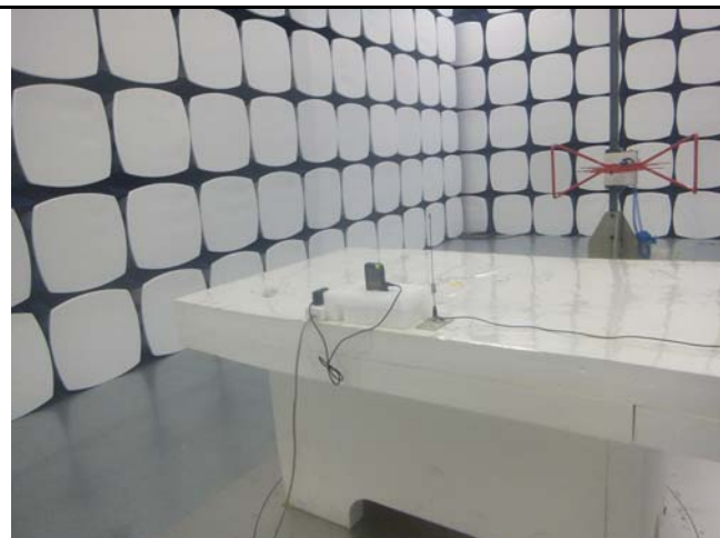
Radiated Spurious Emissions Test Setup Below 1GHz
