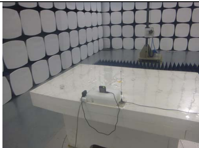
Radiated Spurious Emissions Test Setup Above 1GHz
