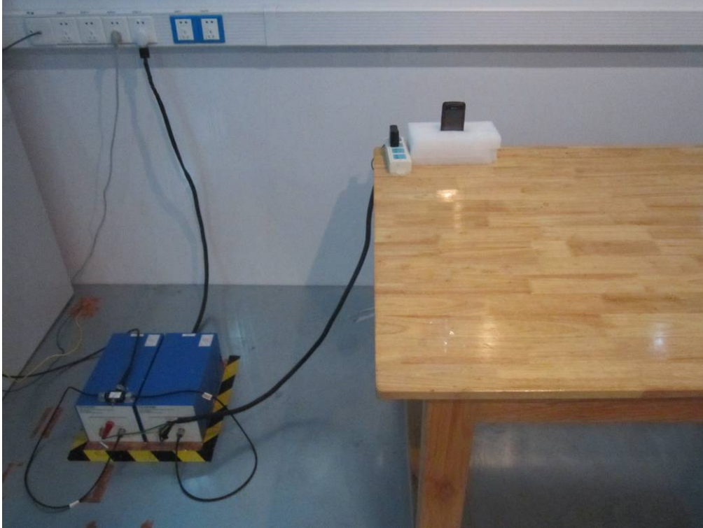
Conducted Emissions Test Setup Front View
