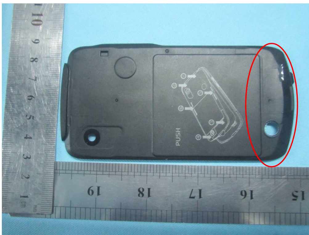
GSM/UMTS Antenna View
