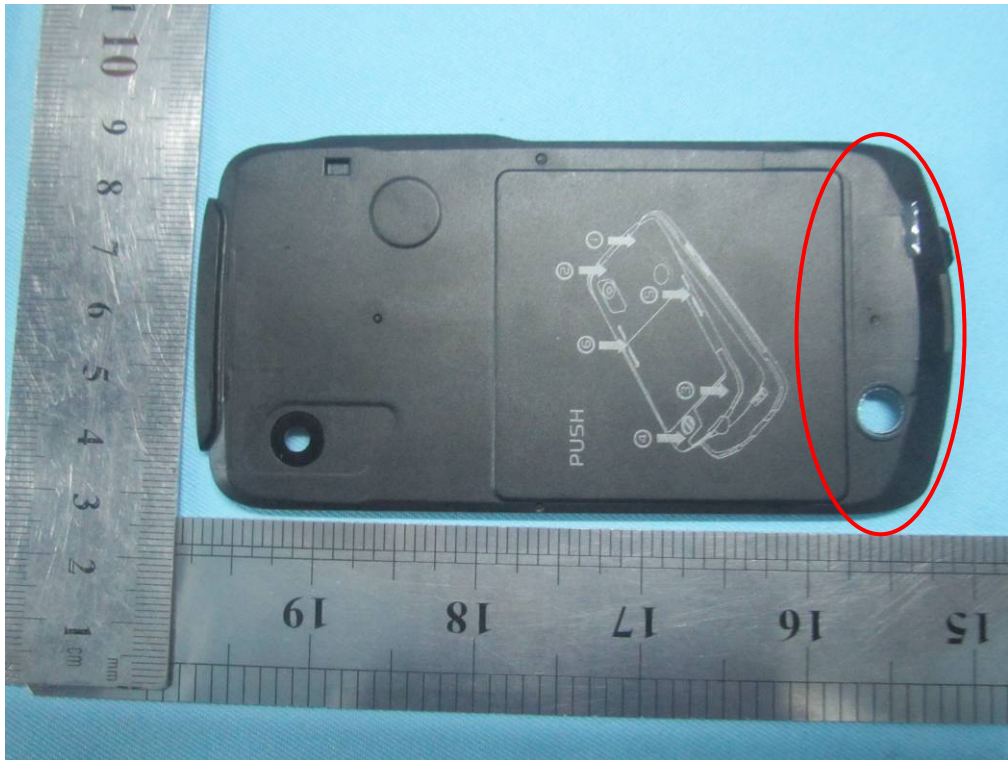
GSM/UMTS Antenna View
